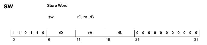
Stores the contents of register rD, into the word aligned memory location that results from adding the contents of registers rA and rB.
